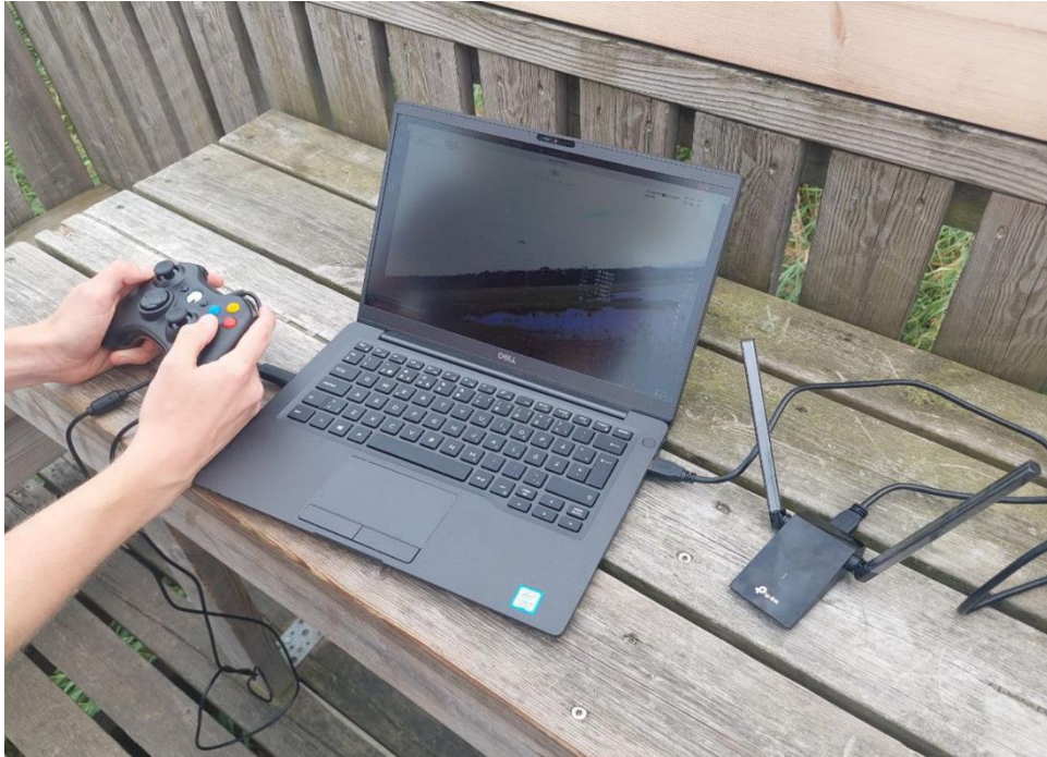
Figure 23. The ground station running OpenHD and QOpenHD where the system can be controlled from
